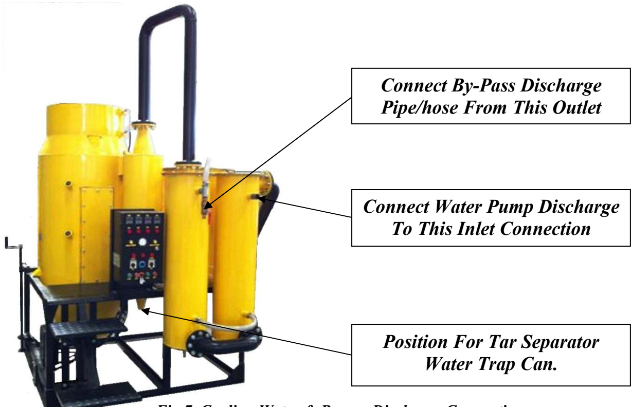
Fig 7. Cooling Water & Bypass Discharge Connection
